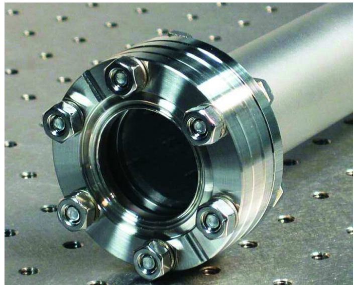
Figure 8. The end port with Viton gasket
